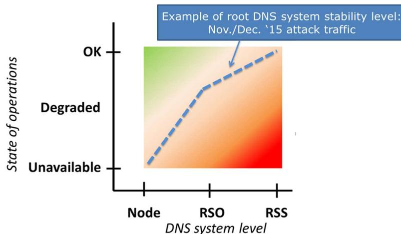
Figure 5: Granularity levels of root DNS system stability
