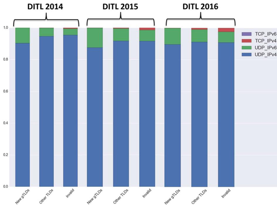
**Figure 11: UDP/TCP and IPv4/IPv6 distribution**
